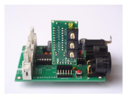
After the LEDs on each card flash, the address is saved. It is stored in the non-volatile memory, the eeprom, and will therefore be preserved after extinction of the arpschuino.
